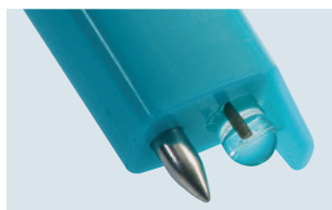
testo 206-pH1: pH1 probe head for liquids
